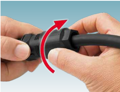
4. Place the union nut on the contact carrier and tighten it until it stops or use the specified torque for tightening.
