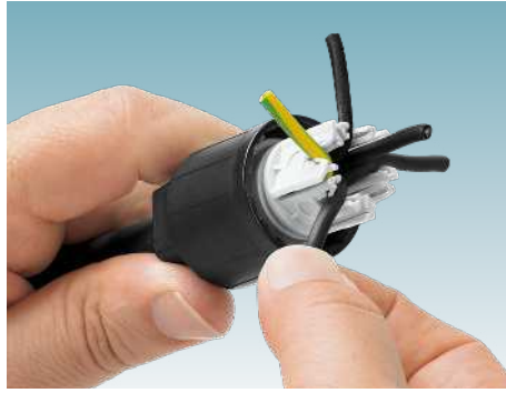
2. Insert the wires into the QUICKON nut and snap into the marked wire guides (1, 2, 3. ...).
